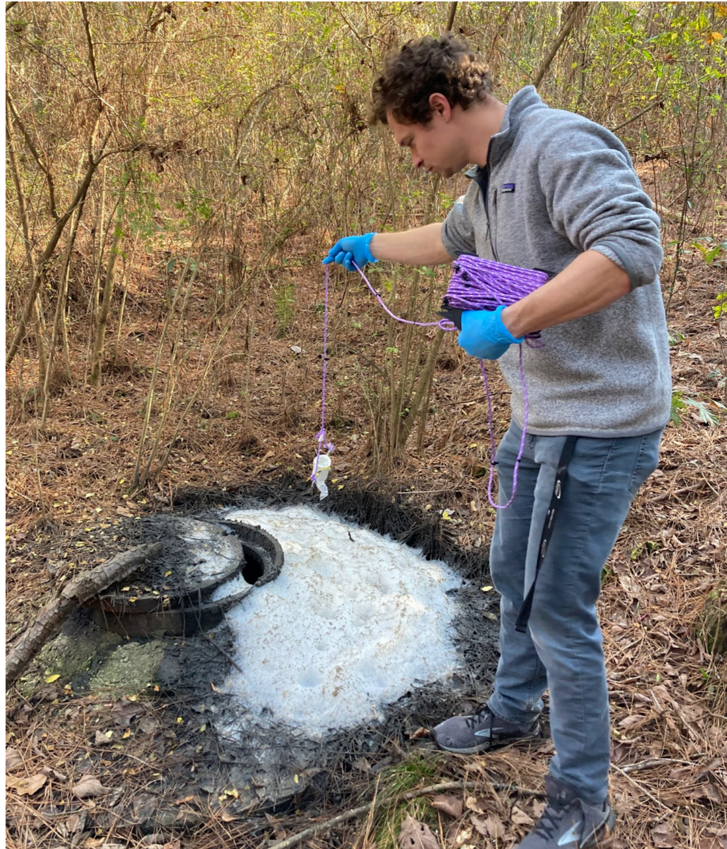
Baykeeper Cade Kistler investigates a sewage overflow to document whether bacteria levels exceed compliance. Sewage spills are a chronic issue for the Mobile Bay area and a major source of pathogen pollution in waterways when untreated waste enters the environment.
